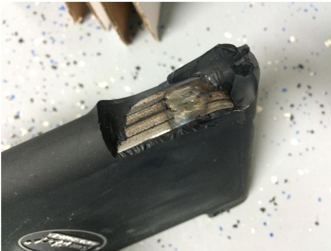
18. Even the weights that had not yet broken appeared cracked and on the verge of breaking.
