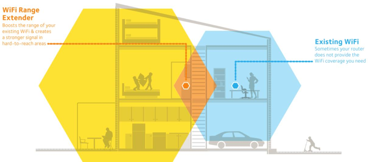
10. As the text in the diagram indicates, the blue hexagon represents the consumer's existing WiFi network. The yellow hexagon is Netgear's representation of the additional range the WiFi network will have when a Range Extender is used.
