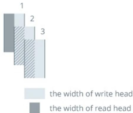
13. SMR thus allows for low-cost, high-capacity HDDs.<sup>7</sup> “However, if new (or modified) data needs to be placed near existing data, the drive will have to overwrite the neighboring shingled tracks ... That makes [SMR] drive[s] significantly slower at writing tasks, especially for random writes.”<sup>8</sup>
