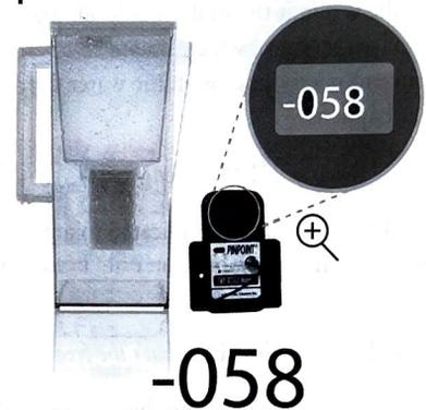
If the number value displayed by the ORP meter is positive (above zero) then the water has oxidizing potential.
