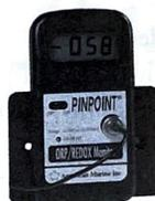
This can easily be proven with something called an ORP meter, which stands for Oxidation Reduction Potential. This device actually measures (in number value) how much a liquid either *reduces* the potential for oxidation, or *creates* oxidation.
